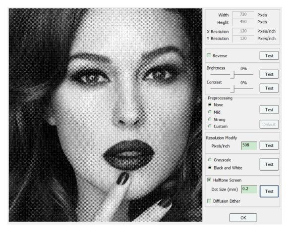
Here, you can reverse the color of the image and change the brightness and contrast of the image. In order to improve the engraving effect, an image preprocessing function is provided to enhance the image contrast effect. If it is black-and-white engraving, we recommend checking the dot or scatter diagram processing. The recommended image resolution is 300 or above.
